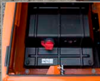
Battery cut-off switch
